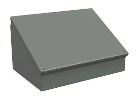
Wiegmann operator consolet, NEMA 12/13, 12 x 16 x 9in (HxWxD), desktop or pedestal mount, carbon steel, ANSI 61 gray, powder coat finish.
