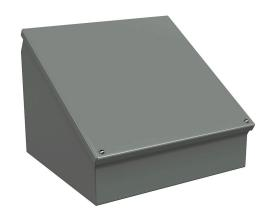
Wiegmann operator consolet, NEMA 12/13, 12 x 12 x 9in (HxWxD), desktop or pedestal mount, carbon steel, ANSI 61 gray, powder coat finish.
