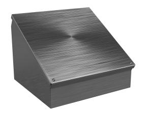
Wiegmann operator consolet, NEMA 4/4X/12/13,  $12 \times 12 \times 9$ in (HxWxD), desktop or pedestal mount, 304 stainless steel, No. 3 intermediate polished finish.
