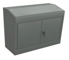
Wiegmann operator console, NEMA 12/13, 36 x 48 x 24in (HxWxD), freestanding, carbon steel, ANSI 61 gray, powder coat finish, flush double-door, 3-point keylocking handle.
