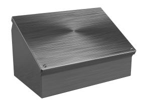
Wiegmann operator consolet, NEMA 4/4X/12/13, 8 x 12 x 7in (HxWxD), desktop or pedestal mount, 304 stainless steel, No. 3 intermediate polished finish.
