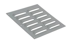
Wiegmann louver vent, 7.87 x 7.50in (HxW), carbon steel, ANSI 61 gray, polyester powder finish, 6.62 x 6.25in (HxW) cutout, for ventilation of metal enclosure. Mounting hardware included.
