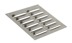
Wiegmann louver vent,  $7.87 \times 7.50$ in (HxW), 316 stainless steel,  $6.62 \times 6.25$ in (HxW) cutout, for ventilation of metal enclosure. Mounting hardware included.
