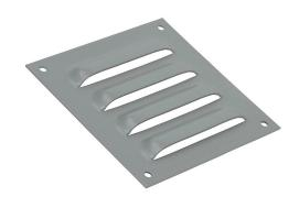
Wiegmann louver vent, 5.62 x 5.50in (HxW), carbon steel, ANSI 61 gray, polyester powder finish, 4.37 x 4.25in (HxW) cutout, for ventilation of metal enclosure. Mounting hardware included.
