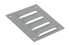
Wiegmann louver vent, 4.75 x 4.50in (HxW), carbon steel, ANSI 61 gray, polyester powder finish, 3.50 x 3.25in (HxW) cutout, for ventilation of metal enclosure. Mounting hardware included.
