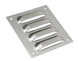
Wiegmann louver vent,  $4.75 \times 4.50$ in (HxW), 316 stainless steel,  $3.50 \times 3.25$ in (HxW) cutout, for ventilation of metal enclosure. Mounting hardware included.
