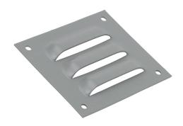
Wiegmann louver vent, 3.87 x 4.50in (HxW), carbon steel, ANSI 61 gray, polyester powder finish, 2.62 x 3.25in (HxW) cutout, for ventilation of metal enclosure. Mounting hardware included.
