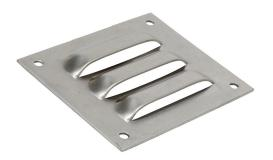
Wiegmann louver vent, 3.87 x 4.50in (HxW), 316 stainless steel, 2.62 x 3.25in (HxW) cutout, for ventilation of metal enclosure. Mounting hardware included.
