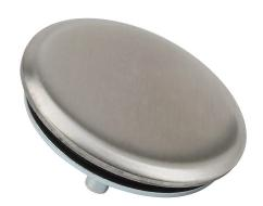
Wiegmann hole seal, 1in conduit, 304 stainless steel, grained finish, oil-resistant gasket. For use with stainless steel enclosures.
