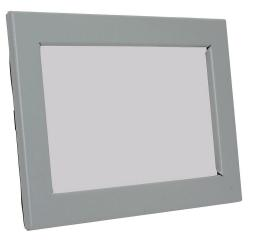
Wiegmann enclosure window, 9.00 x 5.50in window, Makrolon polycarbonate, 11.50 x 8.00in frame, carbon steel, ANSI 61 gray, polyester powder finish, oil-tight closed-cell gasket. For use with indoor NEMA 12 enclosures. Mounting hardware included.
