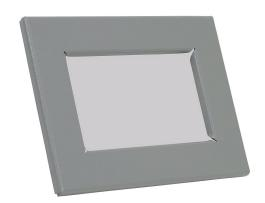
Wiegmann enclosure window, 5.00 x 3.00in window, Makrolon polycarbonate, 7.50 x 5.50in frame, carbon steel, ANSI 61 gray, polyester powder finish, oil-tight closed-cell gasket. For use with indoor NEMA 12 enclosures. Mounting hardware included.
