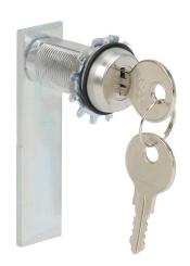
Wiegmann enclosure latch, keylocking, 1/4-turn semi-flush, 1-point, plated steel. For use with single-door NEMA 4 and NEMA 12 enclosures. (2) keys included.
