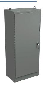
Wiegmann disconnect enclosure, NEMA 12, right flange, 90 x 39 x 24in (HxWxD), freestanding, carbon steel, ANSI 61 gray, powder coat finish, single-door, 3-point padlocking handle, subpanel included.
