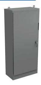
Wiegmann disconnect enclosure, NEMA 12, right flange, 90 x 39 x 20in (HxWxD), freestanding, carbon steel, ANSI 61 gray, powder coat finish, single-door, 3-point padlocking handle, subpanel included.
