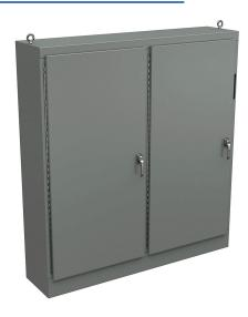
Wiegmann disconnect enclosure, NEMA 12, right flange, 84 x 77 x 18in (HxWxD), freestanding, carbon steel, ANSI 61 gray, powder coat finish, 2-door, 3-point padlocking handle, subpanel included.
