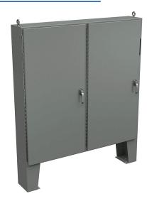
Wiegmann disconnect enclosure, NEMA 12, right flange, 72 x 73 x 12in (HxWxD), floor mount, carbon steel, ANSI 61 gray, powder coat finish, 2-door, 3-point padlocking handle, purchase subpanel separately.
