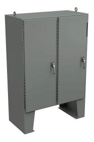
Wiegmann disconnect enclosure, NEMA 12, right flange, 60 x 49 x 24in (HxWxD), floor mount, carbon steel, ANSI 61 gray, powder coat finish, 2-door, 3-point padlocking handle, purchase subpanel separately.
