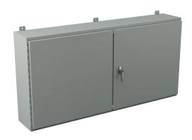
Wiegmann enclosure, NEMA 12, 30 x 60 x 10in (HxWxD), wall mount, carbon steel, ANSI 61 gray, powder coat finish, doubledoor, 3-point keylocking handle.
