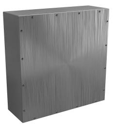
Wiegmann enclosure, NEMA 3/4/4X, 24 x 24 x 8in (HxWxD), wall mount, 304 stainless steel, No. 3 intermediate polished finish, screw cover.
