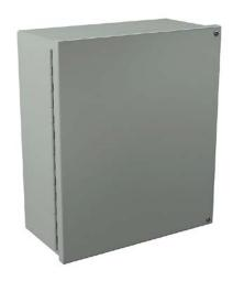
Wiegmann enclosure, NEMA 12/13, 14 x 12 x 6in (HxWxD), wall mount, carbon steel, ANSI 61 gray, powder coat finish, hinged screw cover.
