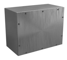
Wiegmann enclosure, NEMA 3/4/4X,  $12 \times 16 \times 8$  in (HxWxD), wall mount, 304 stainless steel, No. 3 intermediate polished finish, screw cover.
