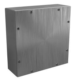
Wiegmann enclosure, NEMA 3/4/4X, 12 x 12 x 4in (HxWxD), wall mount, 304 stainless steel, No. 3 intermediate polished finish, screw cover.
