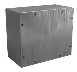
Wiegmann enclosure, NEMA 3/4/4X,  $10 \times 12 \times 6$ in (HxWxD), wall mount, 304 stainless steel, No. 3 intermediate polished finish, screw cover.
