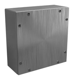
Wiegmann enclosure, NEMA 3/4/4X,  $10 \times 10 \times 4$ in (HxWxD), wall mount, 304 stainless steel, No. 3 intermediate polished finish, screw cover.
