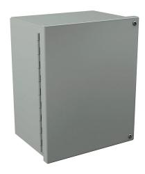
Wiegmann enclosure, NEMA 12/13, 10 x 8 x 6in (HxWxD), wall mount, carbon steel, ANSI 61 gray, powder coat finish, hinged screw cover.
