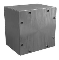
Wiegmann enclosure, NEMA 3/4/4X,  $8 \times 8 \times 6$ in (HxWxD), wall mount, 304 stainless steel, No. 3 intermediate polished finish, screw cover.
