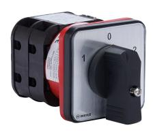
Merz rotary motor reversing cam switch, 2-pole, 600 VAC, 32A, 5kA SCCR, door mount, front operated. Hardware for 4-hole door mounting & black operating handle included.
