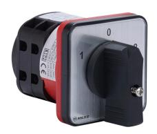
Merz rotary motor reversing cam switch, 2-pole, 600 VAC, 25A, 5kA SCCR, door mount, front operated. Hardware for 4-hole door mounting & black operating handle included.
