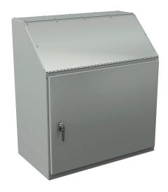
Wiegmann operator console, NEMA 12/13, 40 x 36 x 20in (HxWxD), freestanding, carbon steel, ANSI 61 gray, powder coat finish, single-door, 3-point keylocking handle.
