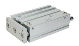
Metal Work pneumatic cylinder, dual guide rod, 63mm bore, 20mm rod diameter, 200mm stroke, double acting, magnetic piston, universal mount.
