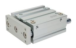
Metal Work pneumatic cylinder, dual guide rod, 63mm bore, 20mm rod diameter, 125mm stroke, double acting, magnetic piston, universal mount.
