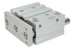
Metal Work pneumatic cylinder, dual guide rod, 63mm bore, 20mm rod diameter, 75mm stroke, double acting, magnetic piston, universal mount.
