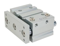
Metal Work pneumatic cylinder, dual guide rod, 63mm bore, 20mm rod diameter, 50mm stroke, double acting, magnetic piston, universal mount.
