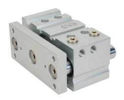
Metal Work pneumatic cylinder, dual guide rod, 63mm bore, 20mm rod diameter, 25mm stroke, double acting, magnetic piston, universal mount.
