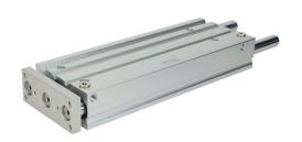
Metal Work pneumatic cylinder, dual guide rod, 50mm bore, 20mm rod diameter, 350mm stroke, double acting, magnetic piston, universal mount.
