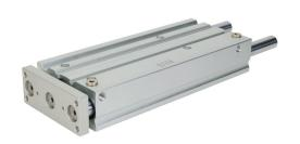
Metal Work pneumatic cylinder, dual guide rod, 50mm bore, 20mm rod diameter, 300mm stroke, double acting, magnetic piston, universal mount.
