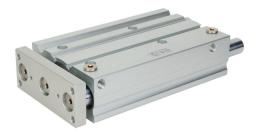
Metal Work pneumatic cylinder, dual guide rod, 50mm bore, 20mm rod diameter, 200mm stroke, double acting, magnetic piston, universal mount.
