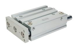
Metal Work pneumatic cylinder, dual guide rod, 50mm bore, 20mm rod diameter, 150mm stroke, double acting, magnetic piston, universal mount.
