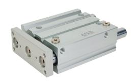
Metal Work pneumatic cylinder, dual guide rod, 50mm bore, 20mm rod diameter, 125mm stroke, double acting, magnetic piston, universal mount.
