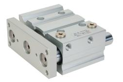
Metal Work pneumatic cylinder, dual guide rod, 50mm bore, 20mm rod diameter, 50mm stroke, double acting, magnetic piston, universal mount.
