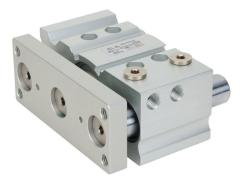
Metal Work pneumatic cylinder, dual guide rod, 50mm bore, 20mm rod diameter, 25mm stroke, double acting, magnetic piston, universal mount.
