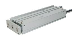
Metal Work pneumatic cylinder, dual guide rod, 40mm bore, 16mm rod diameter, 300mm stroke, double acting, magnetic piston, universal mount.
