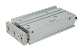
Metal Work pneumatic cylinder, dual guide rod, 40mm bore, 16mm rod diameter, 175mm stroke, double acting, magnetic piston, universal mount.
