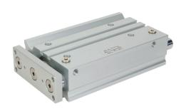
Metal Work pneumatic cylinder, dual guide rod, 40mm bore, 16mm rod diameter, 150mm stroke, double acting, magnetic piston, universal mount.
