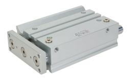
Metal Work pneumatic cylinder, dual guide rod, 40mm bore, 16mm rod diameter, 125mm stroke, double acting, magnetic piston, universal mount.
