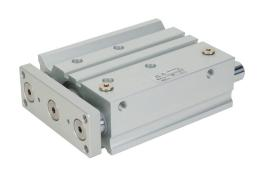
Metal Work pneumatic cylinder, dual guide rod, 40mm bore, 16mm rod diameter, 100mm stroke, double acting, magnetic piston, universal mount.
